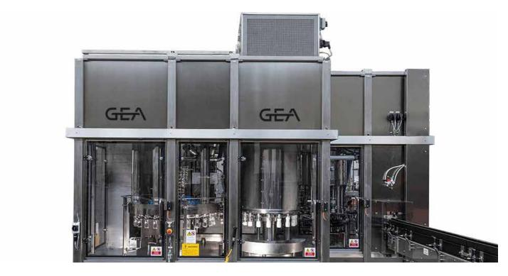
The bottle decontamination treatment is performed in a hygienic cabin where a clean and protected environment is maintained thanks to a topdown laminar flow of sterile air. On the same carousel, both H2O2-based solution injection and subsequent activation with warm air are carried out.
