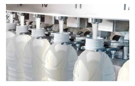
When filling sensitive products it is necessary to combine the most stringent hygiene levels with the highest efficiency and performance. To meet this need GEA designed the Fillstar DX with the aim of achieving completely product scrap-free operation to be used when filling ESL products, and Fillstar FX for aseptic applications.
