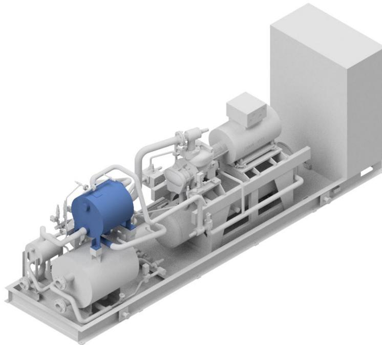
Fig.6: Position of the condenser
