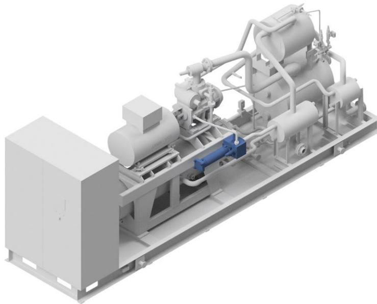
Fig.9: Arrangement of the oil filter system with OMC block
