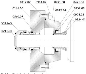
Fig.25: Single flushed mechanical seal
