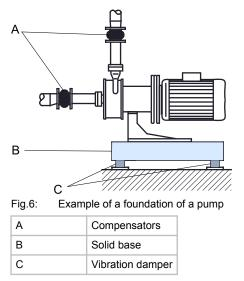
As a guideline, the concrete foundation should be 1.5 times as heavy as the pump.
