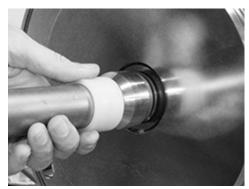
Fig.24: Stationary ring, synthetic material assembly aid
