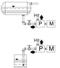
Fig.4: Installation in the piping system top: Inlet operation | bottom: Suction operation | P - Pump | M - Motor
