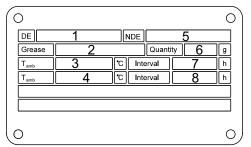
Fig.13: Lubrication information plate of MGE motor (example)
