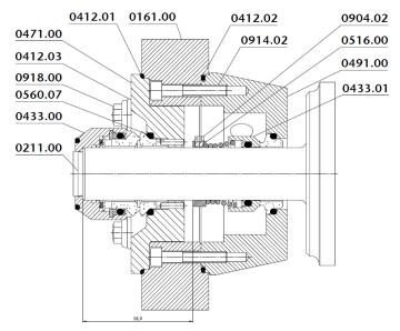
Fig.26: Double mechanical seal tandem
