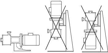
Fig.3: Permissible setups of the pump
