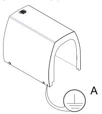
Fig.11: Earthing connection of the motor shroud
