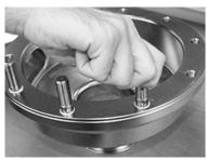
Fig.37: Stud bolts in the HP housing
