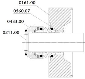
Fig.22: Single mechanical seal
