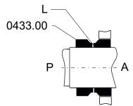
Fig.7:Lubrication film between the sliding surfacesP - Pump side | A - Atmosphere side | L - Lubrication side | 0433.00 - Mechanical seal
