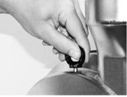
Fig.36: Eye bolt for lifting device
