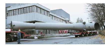
Jet pump for a 4-stage jet vacuum pump for steel degassing suction flow: 1,100 kg/h or 1,387,000  $m^3$ /h, suction pressure abs.: 0.6 mbar
