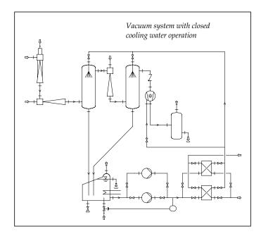
Multi-stage steam jet pumps are employed in the edible oil industry where the product is refined and freed of unwanted aromas by distillation under vacuum (1–5 mbar).
