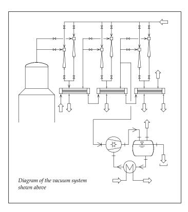
Jet vacuum pumps are used in combination with liquid ring pumps to create vacuum in crude oil distillation columns.
