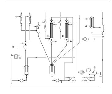
Diagram of a typical product vapour driven jet vacuum pump with mixing and surface condensation
