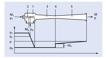
Working principle of a steam jet pump and the pressure differences over the flow path
