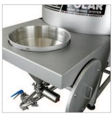
The eductor introduces ingredients directly into the liquid stream, allowing effective mixing without clumping.
