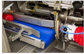
Telescoping conveyor and pneumatic casing brake
