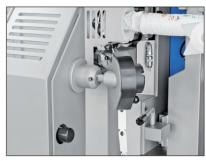
Labels are printed with the printing system and clipped into the exact position via the label dispenser.
