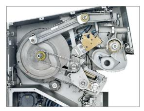
All drive levers are made of solid, stainless cast steel. The electronic clip closing force control "New-Con" increases production reliability
