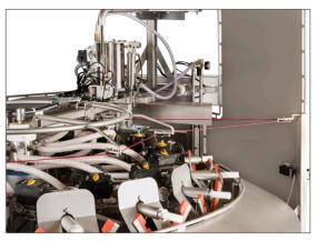
New design features like enlarged clipper guarding screen and red safety cable above the rotating product table enhance operator safety.
