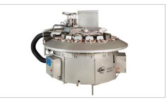
Rota-Matic automatic vacuum packaging system for whole birds, pork shoulders, ground meat chubs, rings, loaves, hams and cheese. Operates at speeds up to 40 packages per minute, with 8 or 16 stations.
