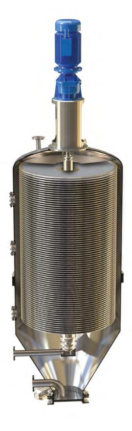
The Funda® Centrifugal Disc Filter is a totally enclosed pressure filter with horizontally arranged, self- supporting filter screens for pre-coat or residue filtration of large quantities of diluted suspensions in an automated, closed system. Heel volume filtration to minimize product losses. Cake washing in cascade operation.
