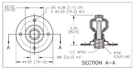
DIMENSIONS ARE SHOWN IN INCHES WITH MILLIMETER EQUIVALENT IN BRACKETS []
