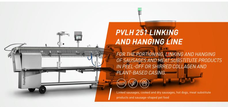
The Handtmann PVLH 251 offers medium-scale and industrial sausage producers an automated production process for the filling, portioning, linking and hanging of cooked and dry sausages in peel-off and collagen casing. Vegan/vegetarian products can also be produced automatically. The production of sausage products from the pet food segment is also possible. The high-performance line comes into its own above all in classic hot dog production and with few product changes.
