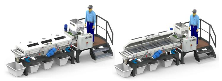
The sieve system is standard equipped with an inlet system, dust hood and control box to make it plug & play. 3 sieves of 600x800mm can be placed inside the frame to sort your product into 4 fractions.
