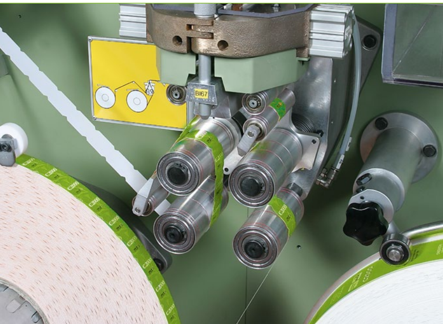
Tag paper reel automatic splicing
