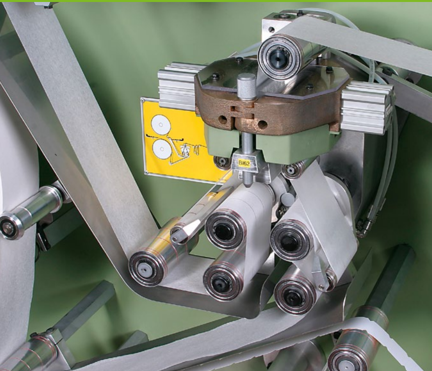
Filter paper reel automatic splicing
