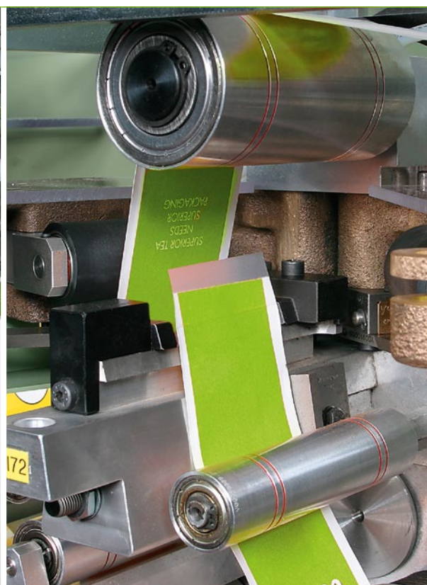
Outer envelope paper reel automatic splicing
