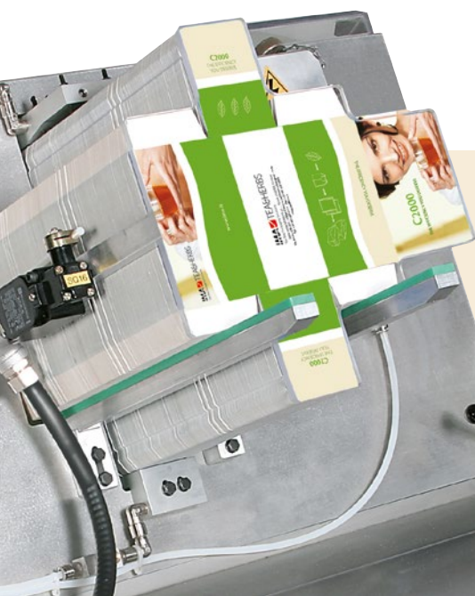
Flat blank collecting and carton erection
