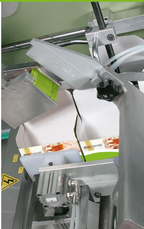
Stack insertion into the cartons
