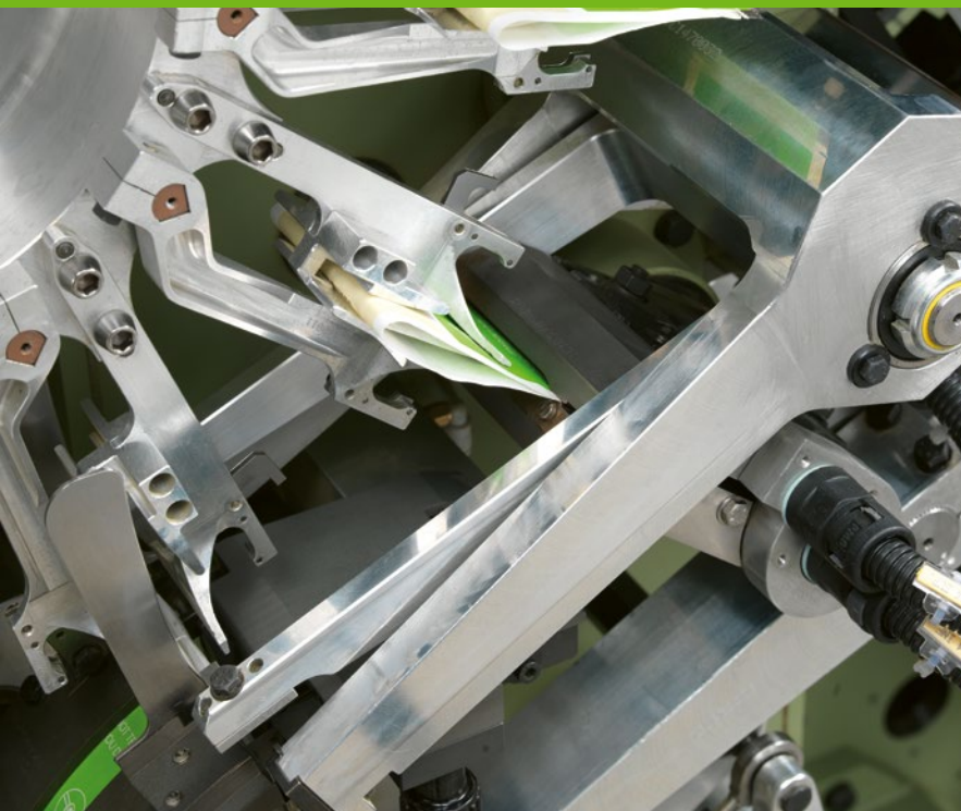
Outer envelope head sealing
