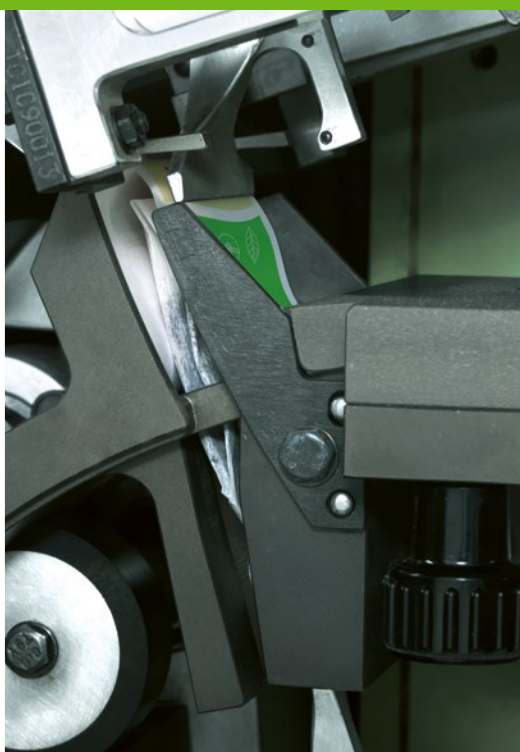
Filter bag overwrapping in outer envelope material
