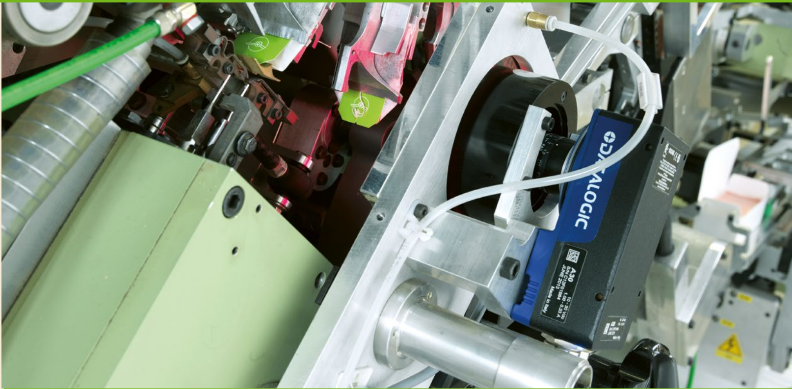
Video camera to control the correct knotting on both filter bag and tag
