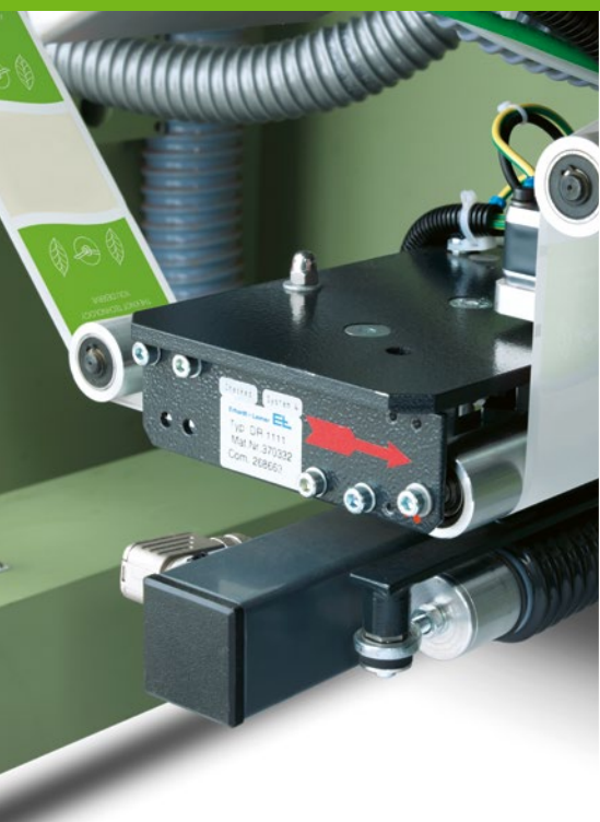
Outer envelope paper alignment control
