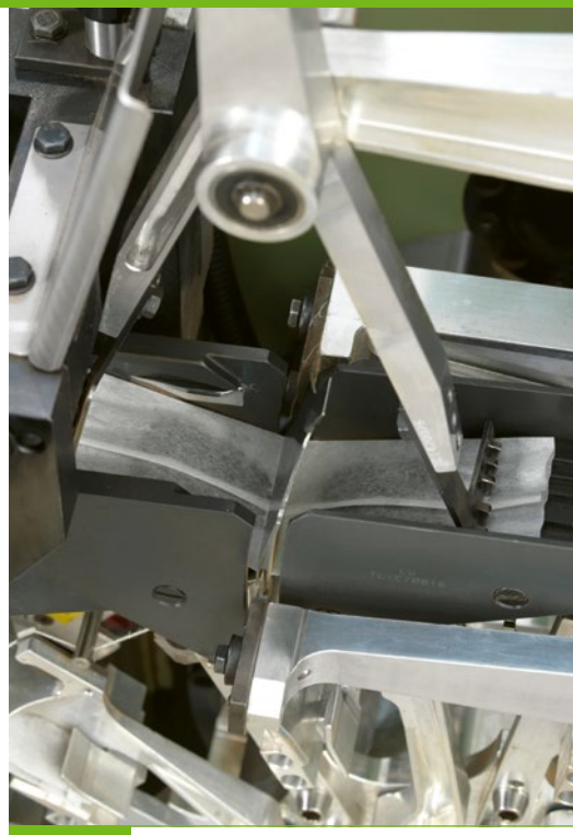
Filter bag tube forming, cutting and erection
