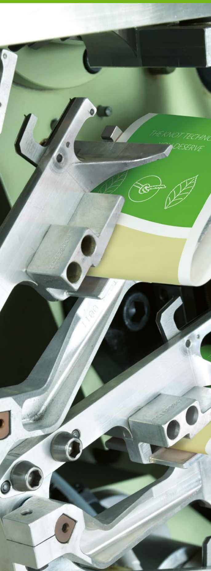
Mechanical single bag rejection
