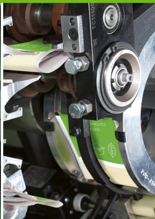
Outer envelope crimping and transfer to stacking unit
