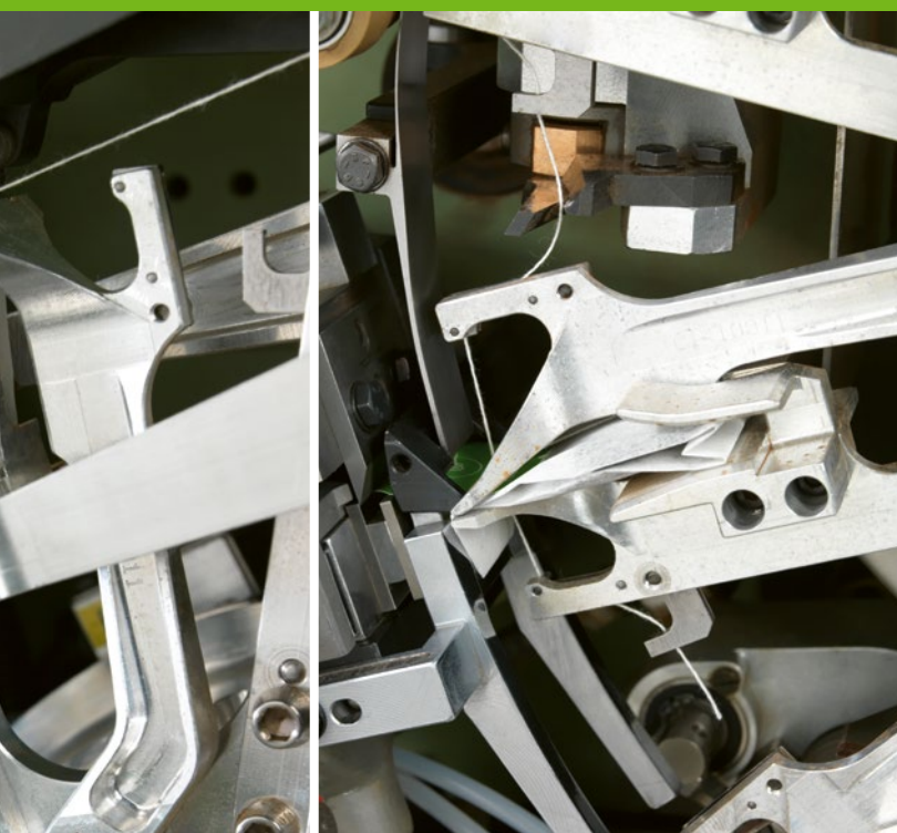
Tag paper feeding, cutting and positioning on the filter bag
