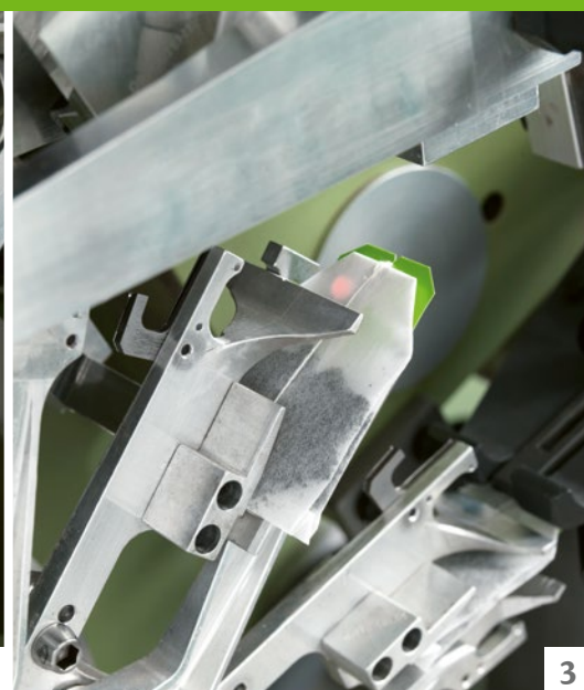
2 KNOTTING knotting on both tag and filter bag
