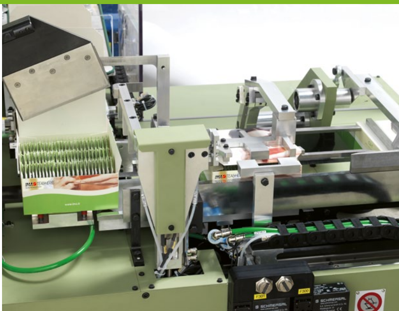
Stack introduction into the carton and flap closing
