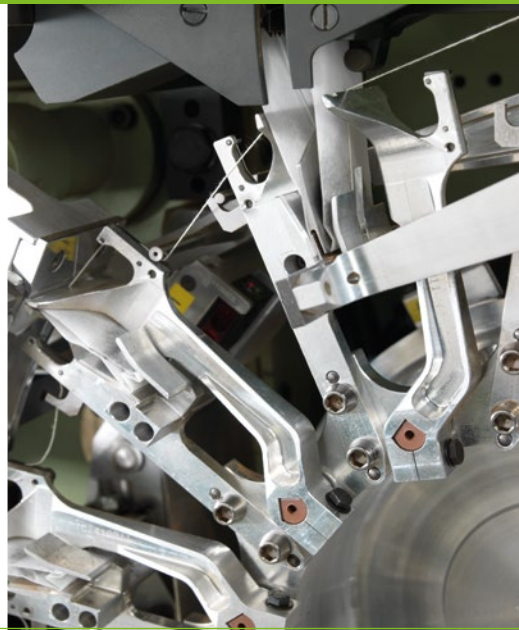
Introduction into the main transfer wheel while the cotton thread is wound around the bag itself
