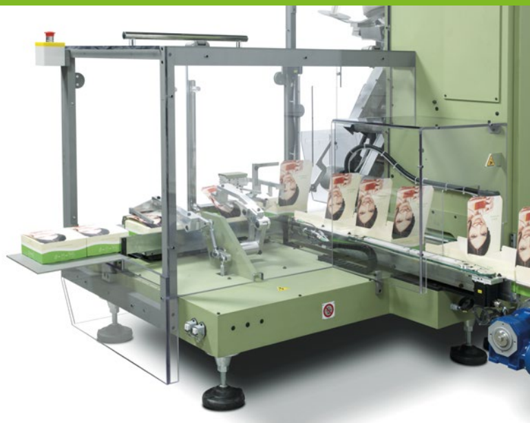
Simplified cartoning attachment for pre-erected cartons
