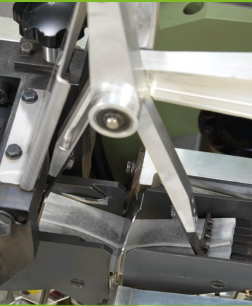
Filter bag tube forming, cutting and erection
