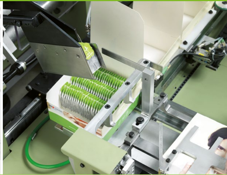
Stack introduction into the pre-erected carton
