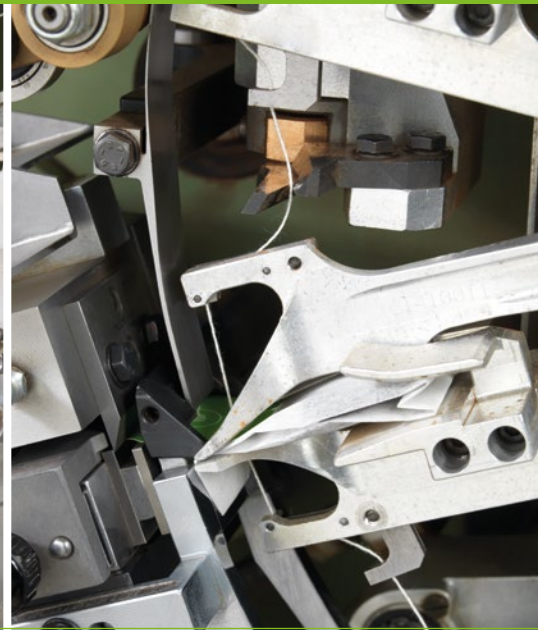
Tag paper feeding, cutting and positioning on the filter bag
