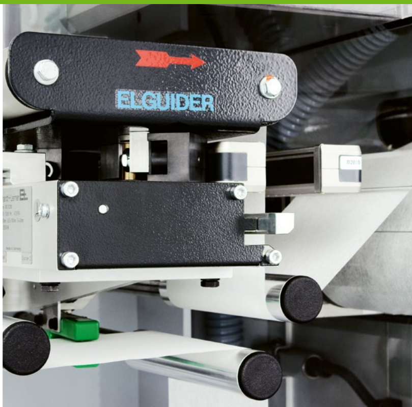
Filter paper alignment
