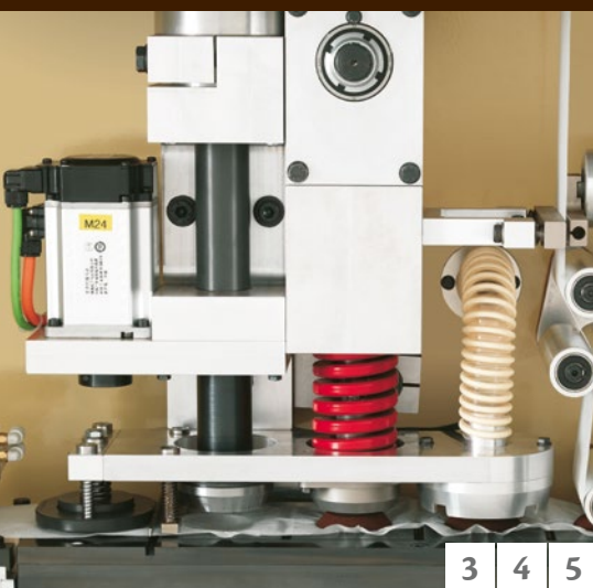
Pod pre-forming, dosing and compacting
