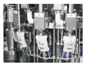
Based on the most modern filling machines, the high speed line for spouted pouches runs with continuous rotary motion. This enables extremely high output and efficiency without sacrificing delicate operations such as sealing, filling and capping. Harmonious movements for limited maintenance and absolute repeatability.
