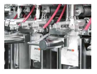
The quality of the container is proportionate to the quality of its seal. Thanks to rotary technology, which enables any operation to be carried out regardless of production speed, the spout is sealed in a single step. This process takes place prior to filling, in a dry controlled environment, in the time required to ensure maximum seal and precision, monitoring and recording all essential parameters such as time, temperature and pressure.
