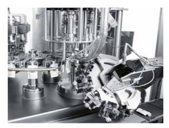
Container handling inside the machine is obtained using the "neck handling" approach, by means of the spout's "rigid" volumes. This firstly enables all operations to be carried out with maximum precision, as the pouch, being "flexible", does not guarantee reliable handling especially at high speeds. In addition, the size changeover is fast, low-cost and offers the freedom to customise and shape the surfaces.
