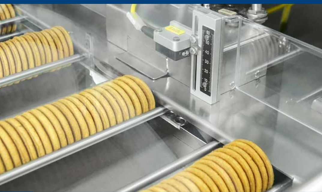
Standard application: single flight bar conveyor
