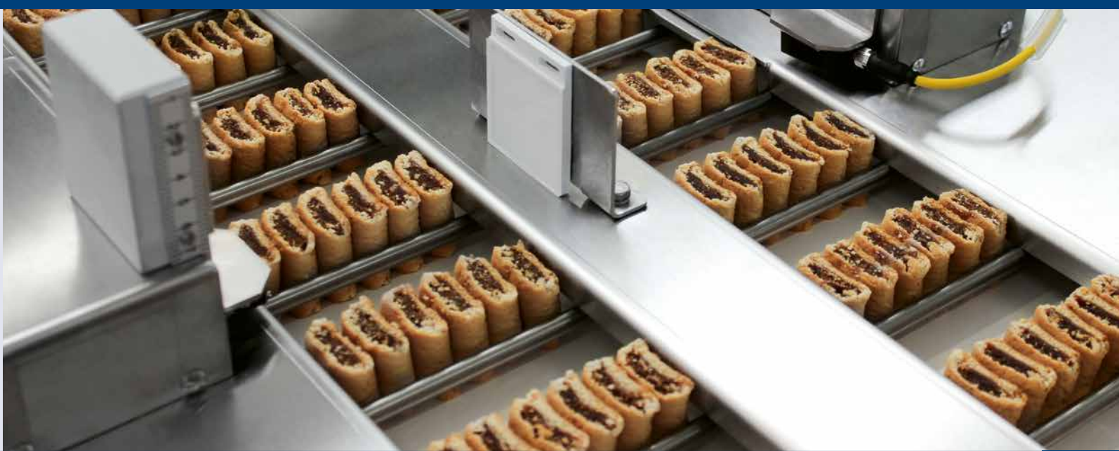
Special application: twin flight bar conveyor complete with moving belt
