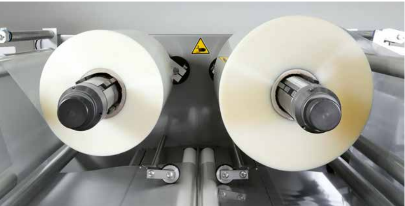
Double reel mounting with automatic film reel splicer
