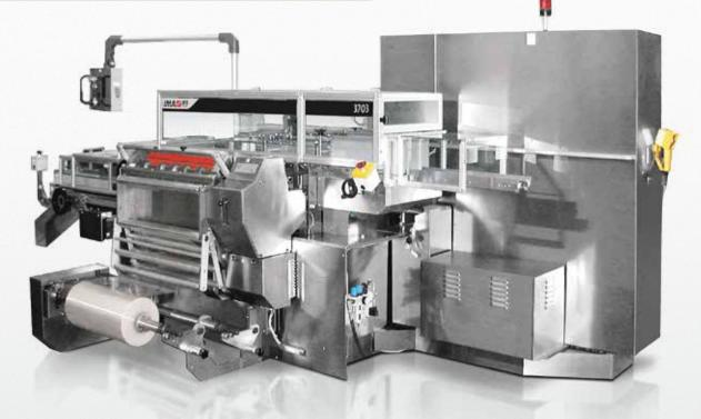
HIGH SPEED WRAPPING AND COLLATING MACHINE: Output speed: Up to 100 Bundles/min.
