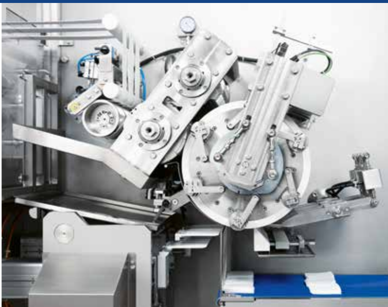
6 clamps cutting and folding drum with servo assisted vertical stacking of single wipes for high precision
