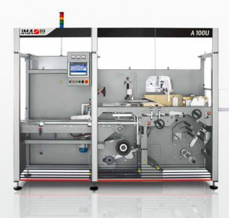
This machine is specifically designed for the food, tea and cosmetic markets, meets the request of reduced overall dimension, accessibility, a very easy size changeover procedure and maximum reliability. It is possible to automatically wrap cartons, trays, and other parallelepiped products with heatsealable materials from reel of cellophane, PP, PVC, ecc.
