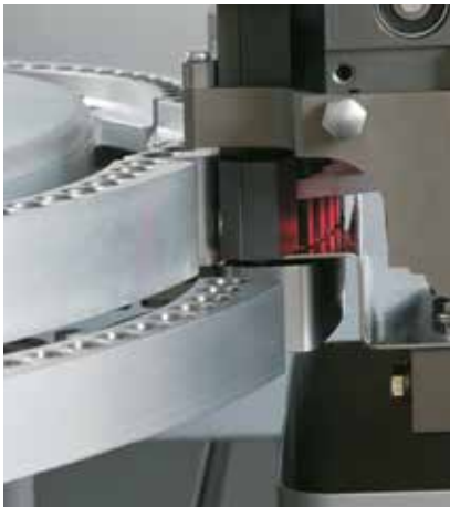
Sensor to check tablet/capsule presence
