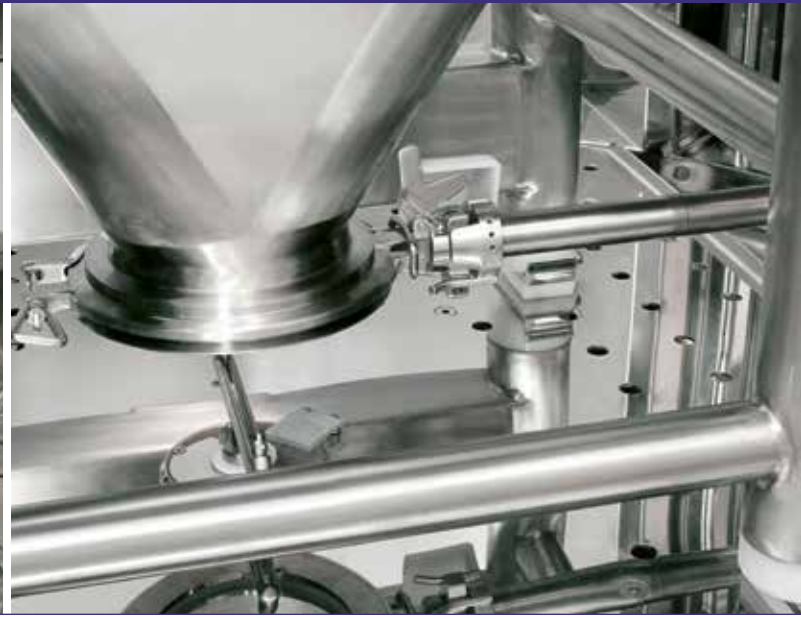
Automatic opening of the lower bin valve
