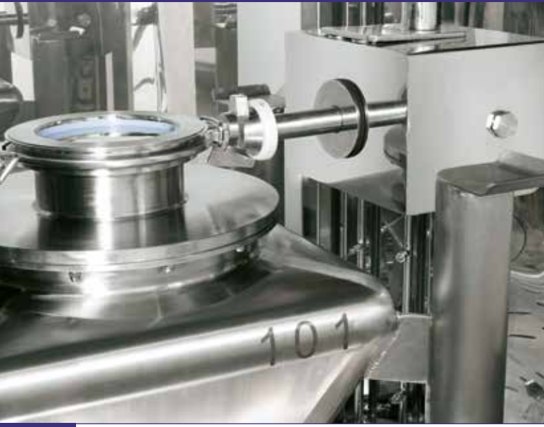
Automatic opening of the upper bin valve
