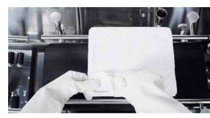
Manual de-lidding and linear removal under isolator
