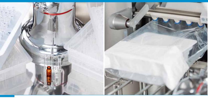
Tub debagging & relevant transfer to the isolated area
