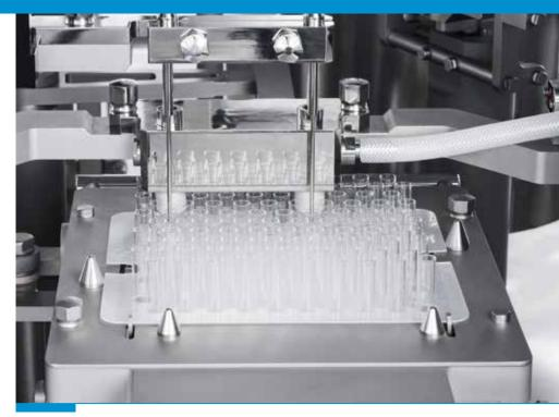
RTU cartridge filling and plugging
