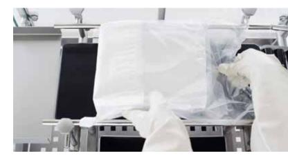
Outer bag manual cutting under Laminar airflow hood
