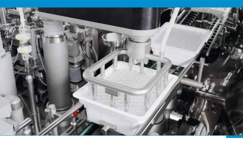
Sterifill RS Series automatic denesting at infeed
