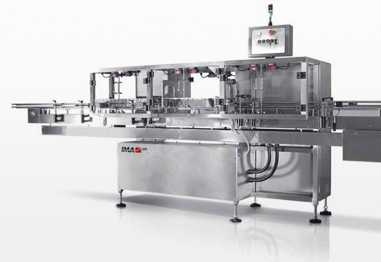
THE IMA SWIFTPACK INLINE BOTTLE CLEANING MACHINE HAS BEEN DESIGNED TO MEET THE HIGHEST LEVEL OF GMP IN KEEPING WITH THE STRINGENT REQUIREMENTS SET BY THE PHARMACEUTICAL INDUSTRY. BOTTLES ARE INTRODUCED INLINE TO THE MACHINE AND ARE INVERTED OVER A SET OF OSCILLATING AIR-JET NOZZLES THAT PENETRATE INSIDE EACH BOTTLE WITH CLEAN AIR. A STATIC ELIMINATION DEVICE IS ALSO IN PLACE TO ASSIST WITH THE REMOVAL OF ANY POSSIBLE DEBRIS FROM WITHIN THE BOTTLE.
