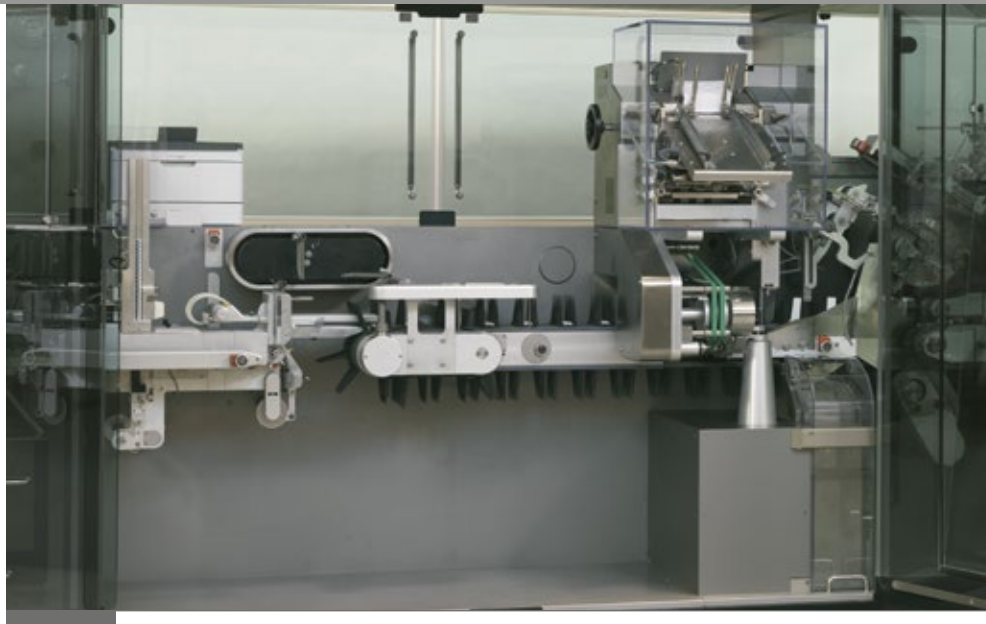
C80HS-A96 / A86 - Connection to the cartoner
