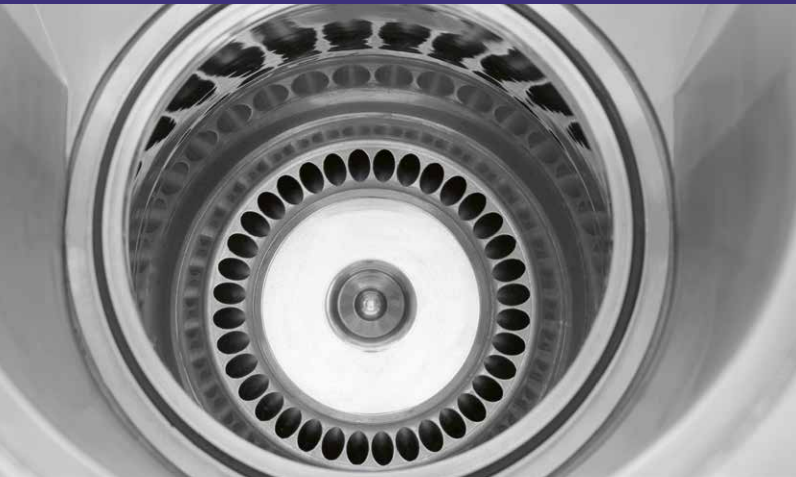
Inner view of the turret and openings of the radial channels for powder feeding to the dies: one feeding channel for each pressing station.
