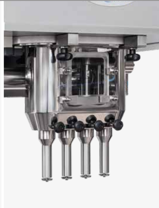
AUGER DOSER for powders, free and non free flowing products
