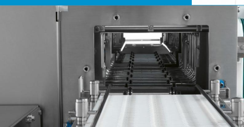
**NEBULA** is an efficient, simple concept which avoids the complexity of NTT systems. It is based on chemical decontamination by HC-VPHP and provides an easily-managed tub or tray infeed process. Whereas NTT systems have a non-negligible impact on line layout, NEBULA is a 3-stage tunnel which simplifies the entire decontamination process, starting from a standard infeed.
