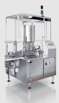
A 3 head rotary capper suitable for speed up to 100 bpm. Machine can handle round or irregular shaped containers, screw or press-on caps. The cap feeder is mounted on a simple electrically adjusted stand complete with an enclosure around the cap feeder for noise reduction, the capper turret is a powered adjustment to accommodate different height bottles.
