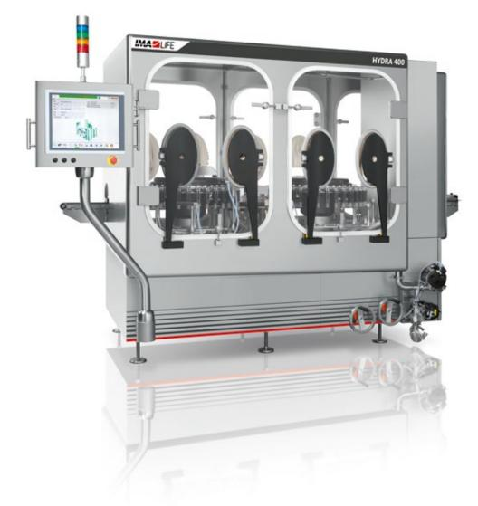
Hydra 400 is designed according to the same criteria as Hydra 100/300, but is fitted with two carousels, one for washing and one for drying, enabling higher speeds.
