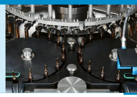
The containers are placed on a conveyor belt which keeps them compact during the loading phase. A scroll gently transfers the containers from the infeed belt to the transport starwheel where they are picked up by the pincers mounted on the central carousel.
