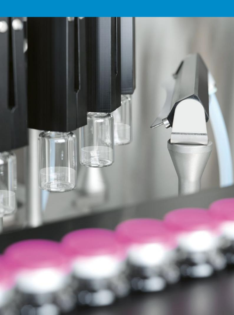
IDEAL FOR COMPLETION OF ASEPTIC PROCESSING LINES, HYDRA 100/300/400 ARE SPECIFICALLY DESIGNED TO PERFORM THE DECONTAMINATION OF EXTERNAL SURFACES OF GLASS OR PLASTIC CYLINDRICAL CONTAINERS (BOTTLES, VIALS, ETC.) WHICH COULD HAVE BEEN POTENTIALLY CONTAMINATED BY THE PRODUCT DURING THE FILLING PROCESS.
