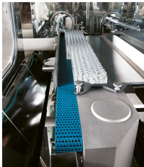
Fixed system integrated with an aseptic filling line under isolator.
