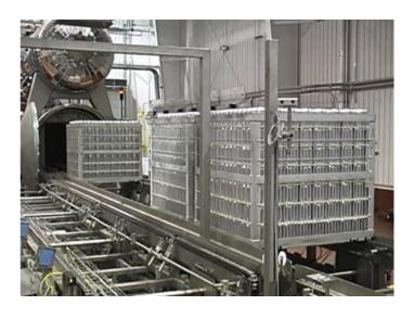
loader to pick up baskets for retorting. A fleet of conveyor-deck AGVs transports baskets from the loader conveyors to the batch retorts for high temperature cooking. Once the sterilization cycle is complete, the retort opens automatically and an AGV is sent for unloading. An AGV is ordered to remove the baskets and deliver them to the unloader or a buffer conveyor. AGVs also transport empty baskets to and from the buffer conveyors.
