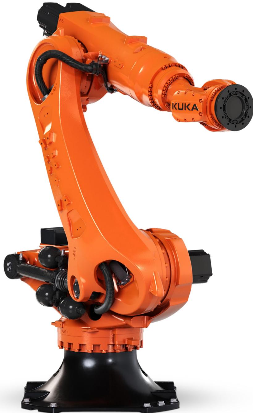
The KR FORTEC is our all-rounder among the heavy-duty robots. It is energy-efficient and dynamic for handling applications in the heavy payload range up to 500 kg. Thanks to its use of our well-known industrial robot concepts, it requires little maintenance when in operation. This gives the robot a high reliability factor in your production.
