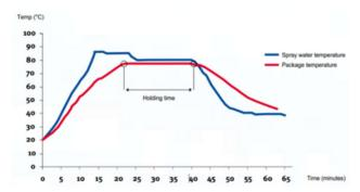
In the diagram, an example is shown of temperatures inside the bottle compared to the temperature of the water sprayed. The overshoot temperature and overshoot time can be set.
