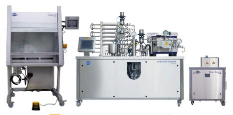
20L/hr HTST/UHT + Homogenizing + Steam Generator + Filling
