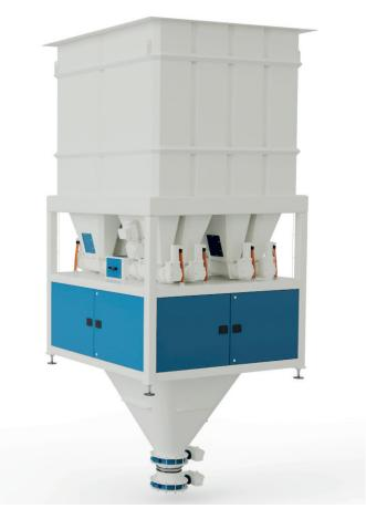
The Micro Dosing Unit (MDU) is a modular build high accuracy dosing system suitable for a wide range of different applications. It is also an easy expandable system in case needed. The MDU consists of a robust and hygienic designed base-frame made of steel box sections with the bin hoppers, dosing equipment and scales fully integrated.
