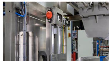
Box lift system to reduce drop distance
