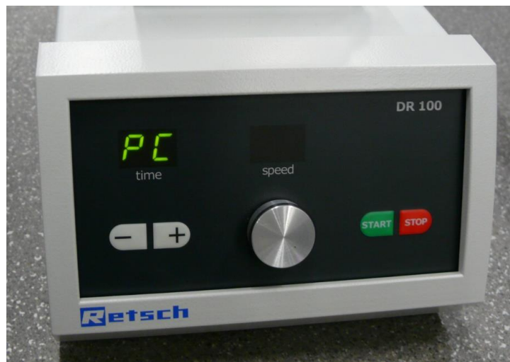
Fig. 30: Display of the feed unit when controlled by the ZM 300
