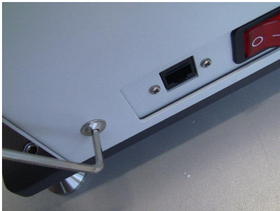
Fig. 5: Remove the rear metal-sheet panel.
