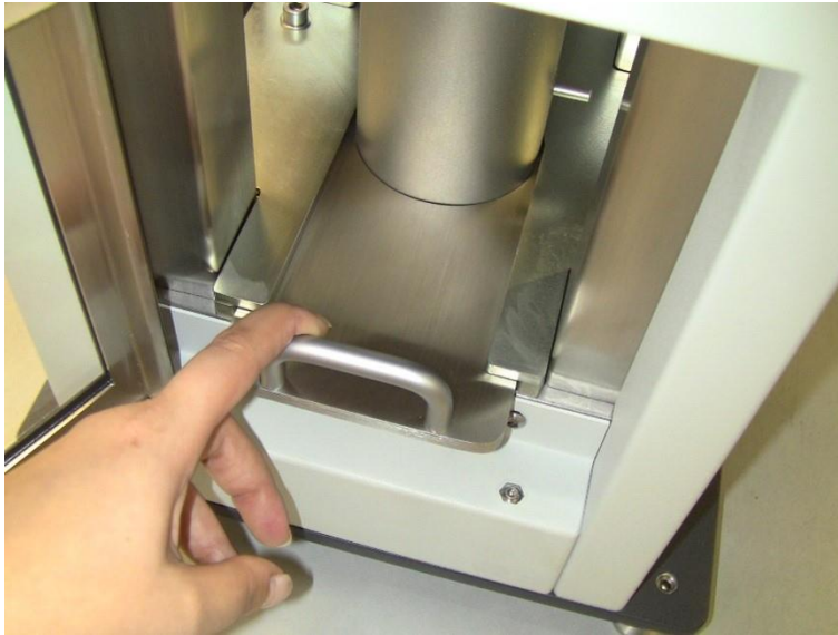
Fig. 8: Pull out the tool sliding tray.
