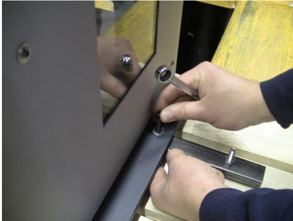
Fig. 4: Loosen the transport aid screws
