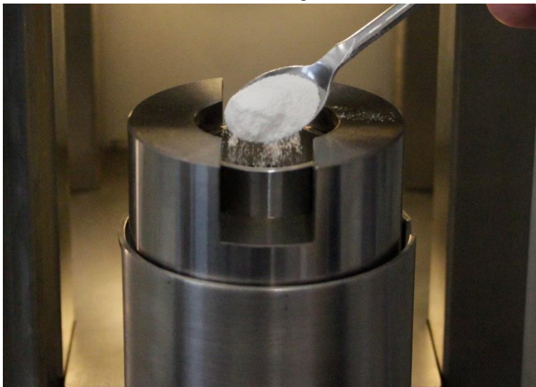
Fig. 25: Fill in the feed material
