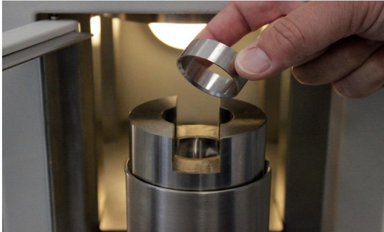
Fig. 24: Insert the steel ring.
