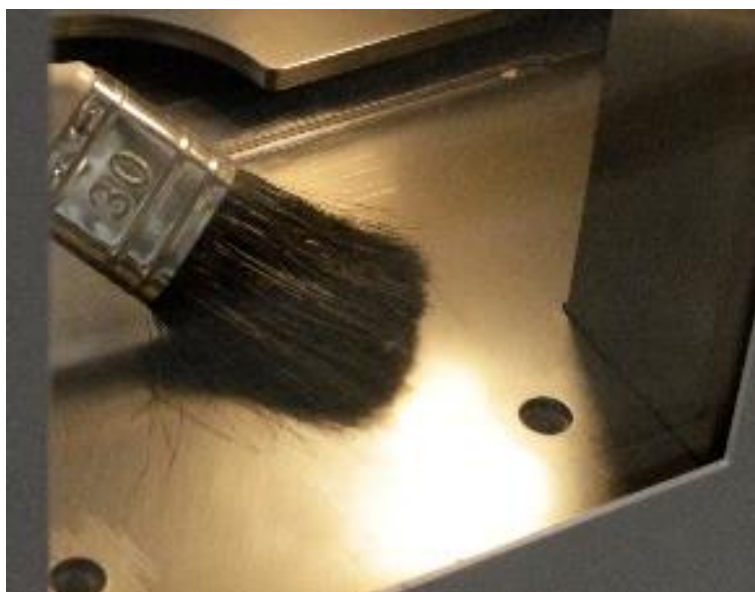
Fig. 42: Clean the pressing chamber.
