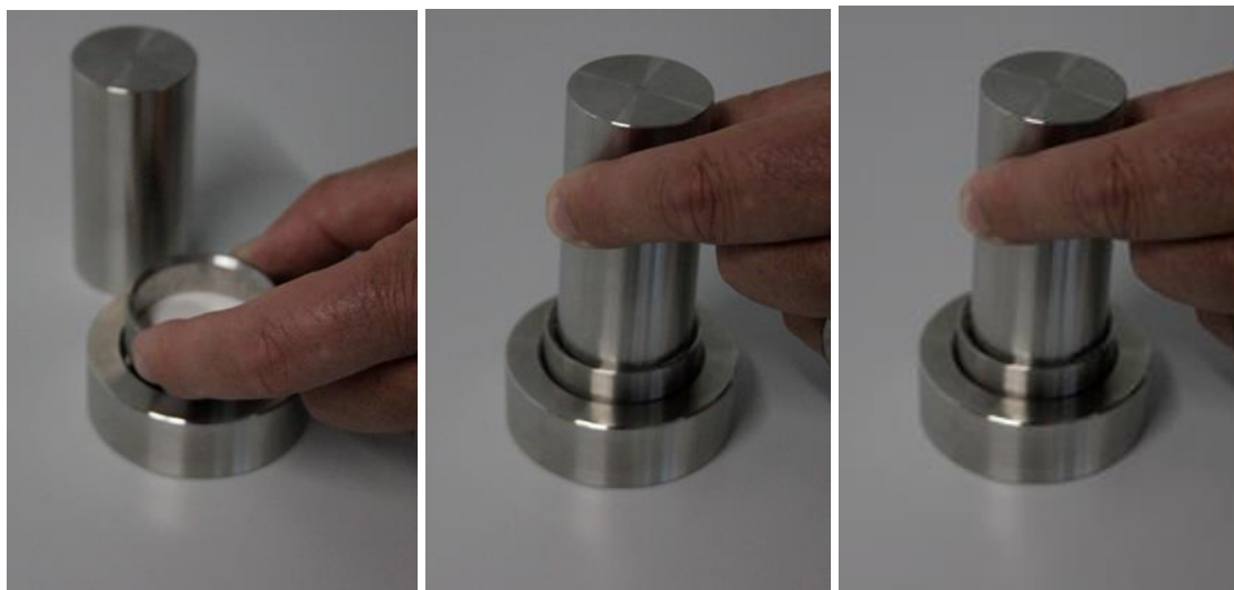
Fig. 26: Remove sample out of the steel ring.
