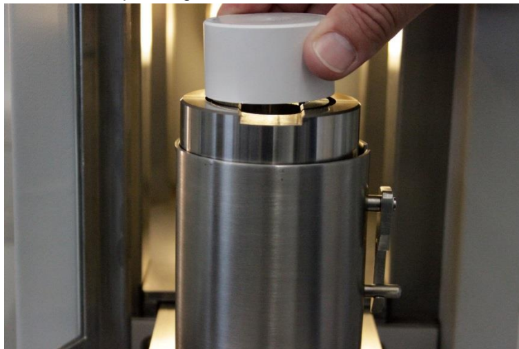
Fig. 18: Put on the pressing-out aid
