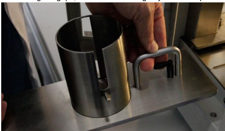
Fig. 39: Remove the tool sliding tray.
