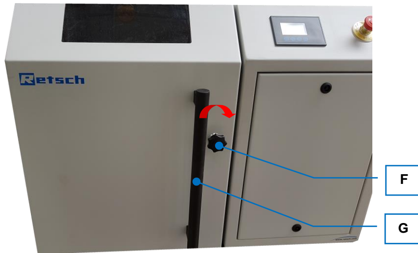
Fig. 11: Closing the housing door
