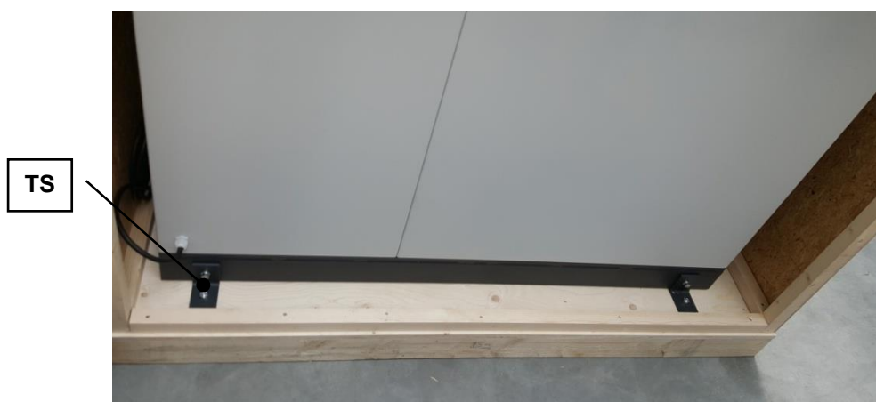
Fig. 1: Unscrewing the transport lock from the transport pallet
