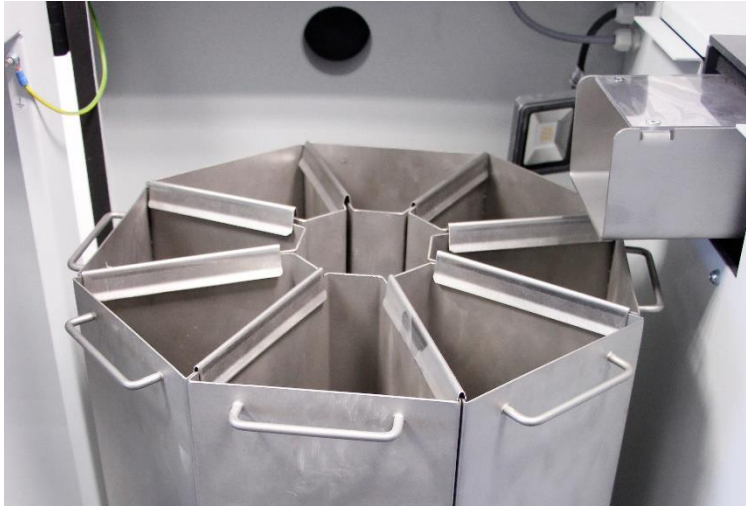
Fig. 3: Machine with inserted vibratory feeder with splashback
