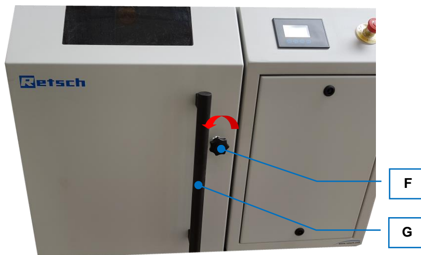
Fig. 10: Opening the housing door
