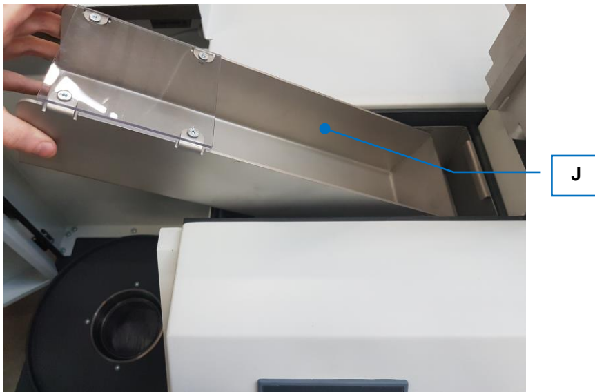
Fig. 15: Inserting the vibratory feeder
