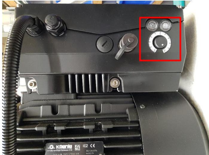
Fig. 18: Rotary control on the motor
