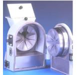
The material sample is crushed by two milling discs coarsely meshed on the inside working against one another in a milling space sealed against dust from the outside. One of these is driven by a powerful and slow moving gear motor.
