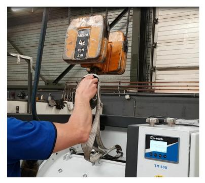
Fig. 31: Securing the drum
