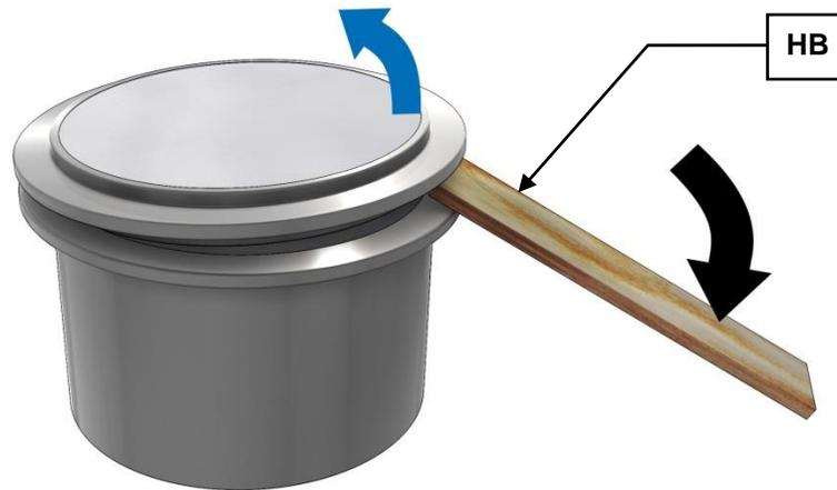
Fig. 28: Prising the grinding jar lid open
