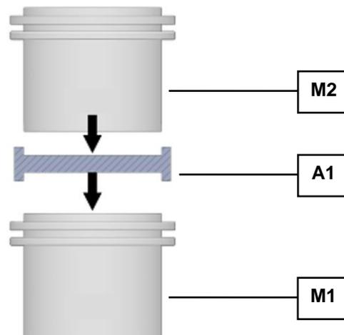
Fig. 24: Stacking grinding jars on the PM 100
