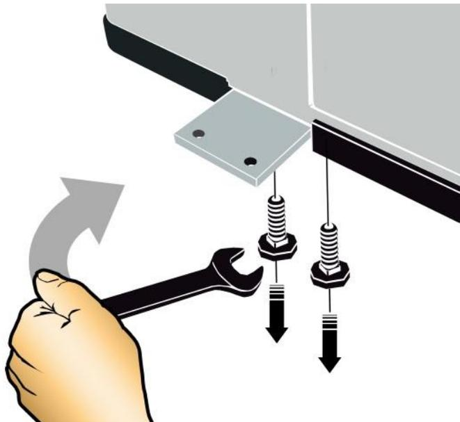
Fig. 4: Removing the transport lock from the device
