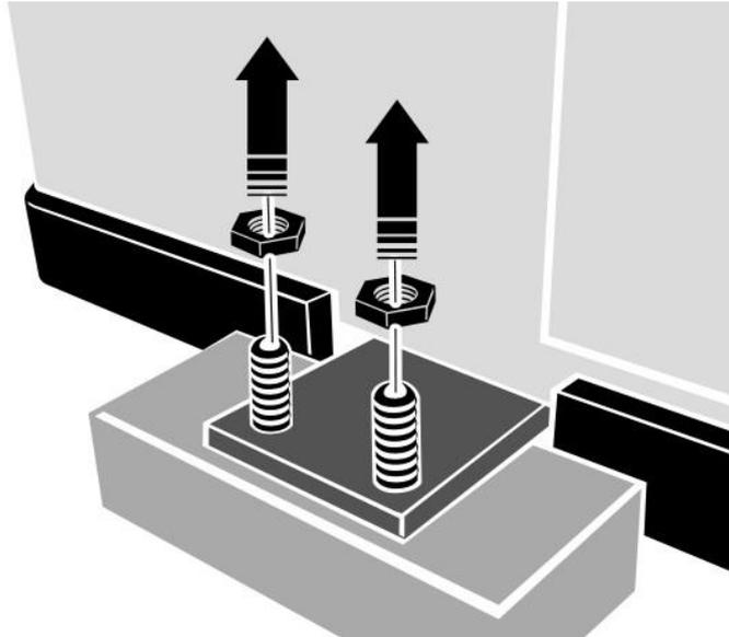
Fig. 3: Unscrewing the transport lock from the transport pallet
