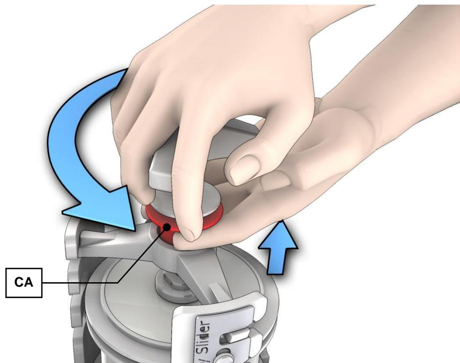
Fig. 20: Releasing the grinding jar clamping mechanism
