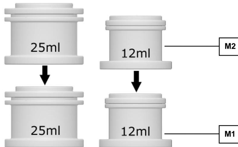
Fig. 25: Stacking the 25 ml and 12 ml grinding jars
