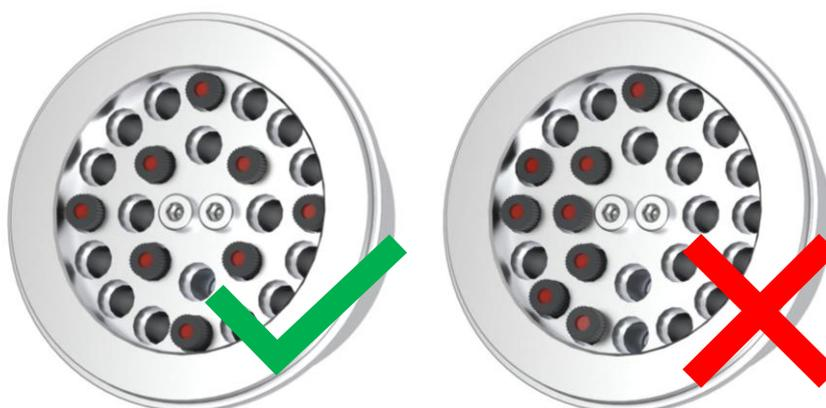
Fig. 35: Permissible arrangement of the glass vials in the adapter
