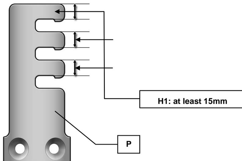
Fig. 41: Wear to the latching bracket
