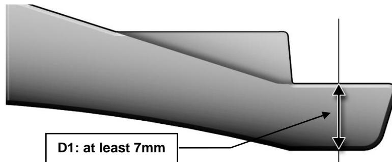
Fig. 39: Wear to the bases of the clamping unit
