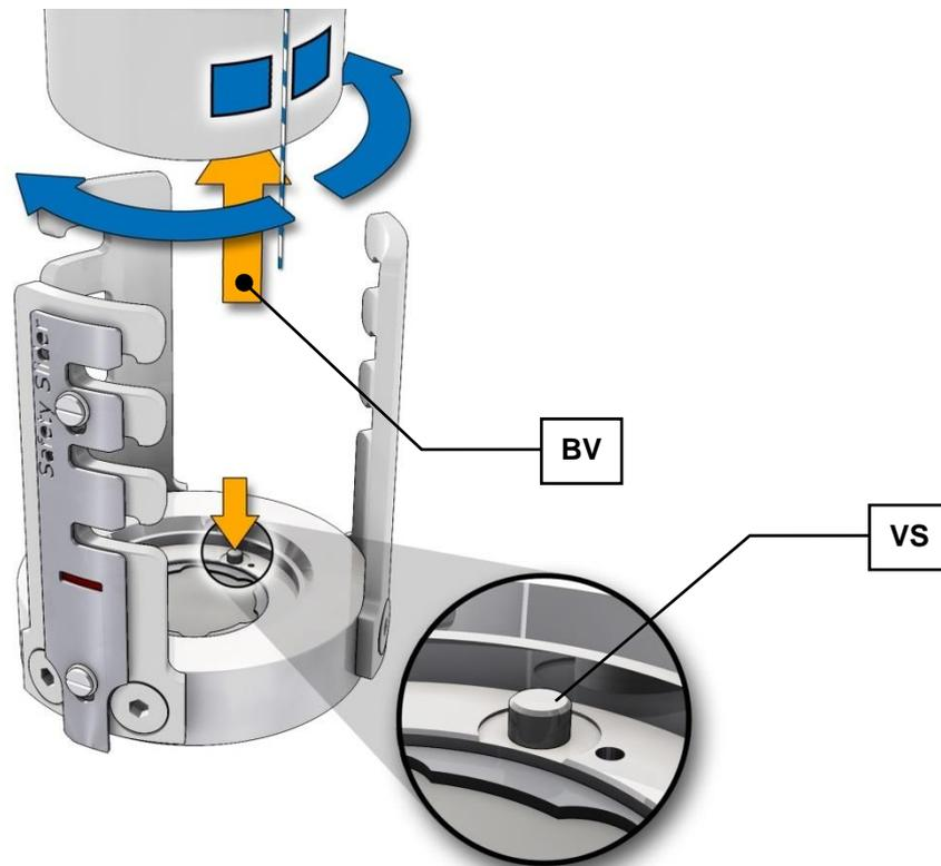
Fig. 27: Anti-rotation device
