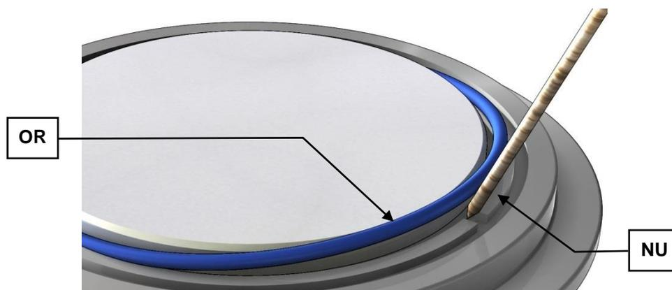
Fig. 30: Removing the O-ring
