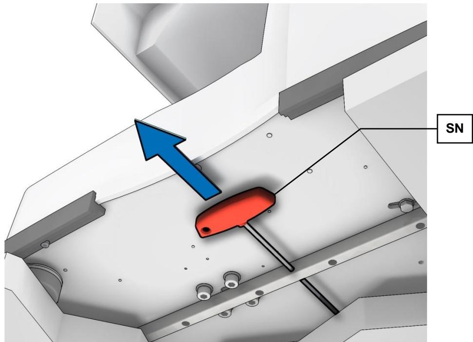
Fig. 12: Storage of key for emergency release
