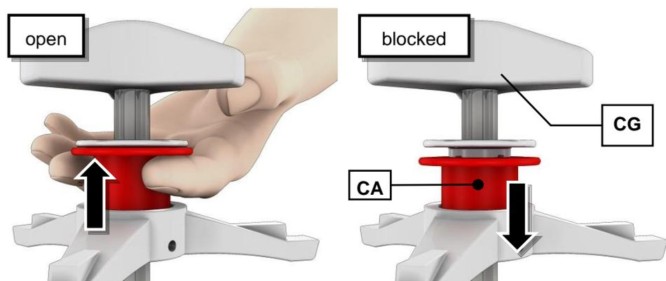
Fig. 17: Function of the locking sleeve
